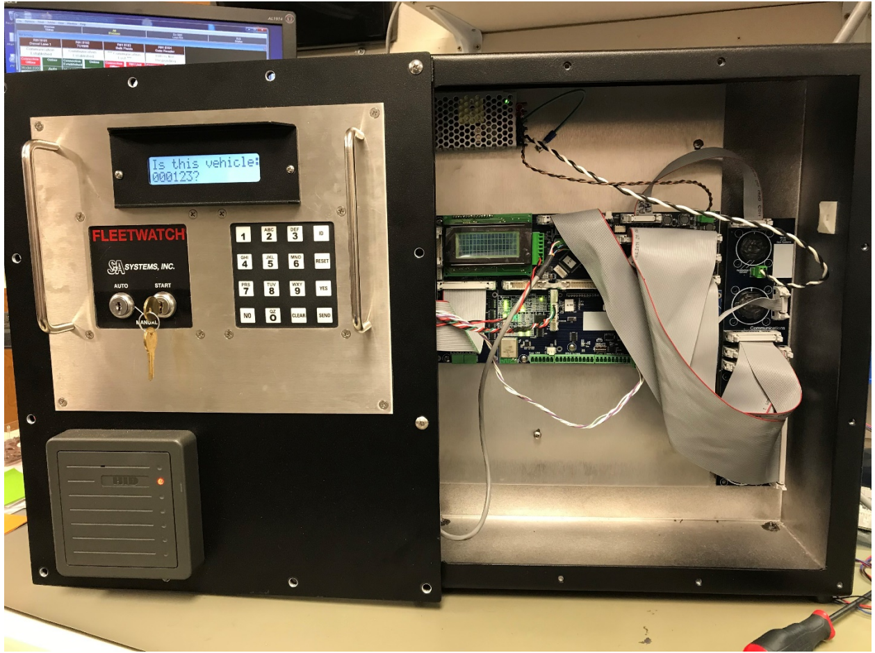
Figure 3: attach the cover in this manner if working on the RIH in its installation location
