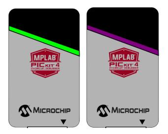
18. After the device LED returns to green, disconnect power then programming cable. Congratulations you have programmed the board successfully! (It is recommended to write the firmware version number (e.g., v1.07) on the board.)
