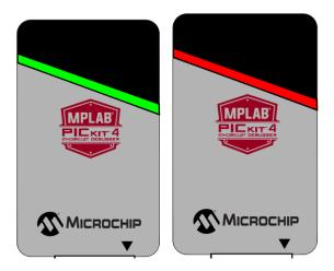
17. When the device LED is green and ready to program, press firmly on the shield logo on the face of the device. The light will flash purple during programming, then back to
